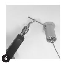
Cut the suspension wire to the desired wire length.
